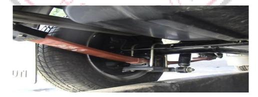
Figure 1 New generation composite leaf springs
